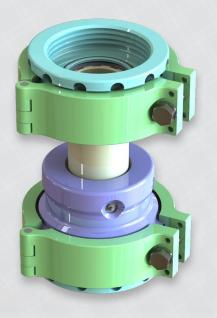
Premium's SDL-75 washpipe cartridge brings an economical hammerless solution to your top drive. The SDL-75 uses standard seals, but unlike conventional washpipes, the seals can be pre-compressed in the housing before installation.
